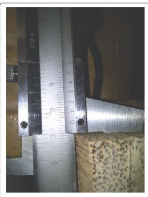
Fig. 7 Tangential swelling test
