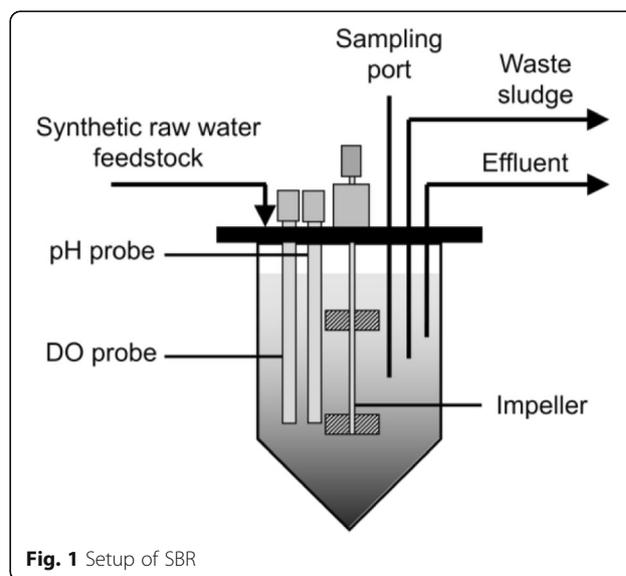
**Fig. 1** Setup of SBR
