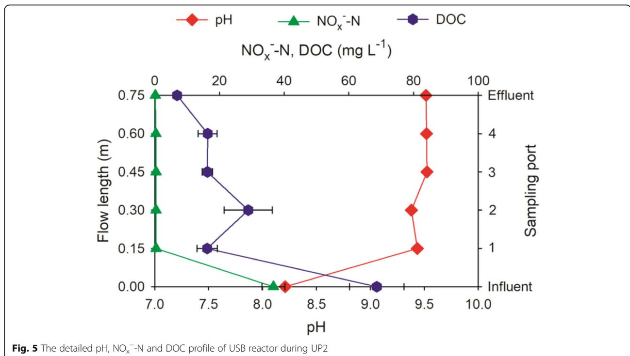
**Fig. 5** The detailed pH, NO<sub>x</sub><sup>-</sup>-N and DOC profile of USB reactor during UP2
