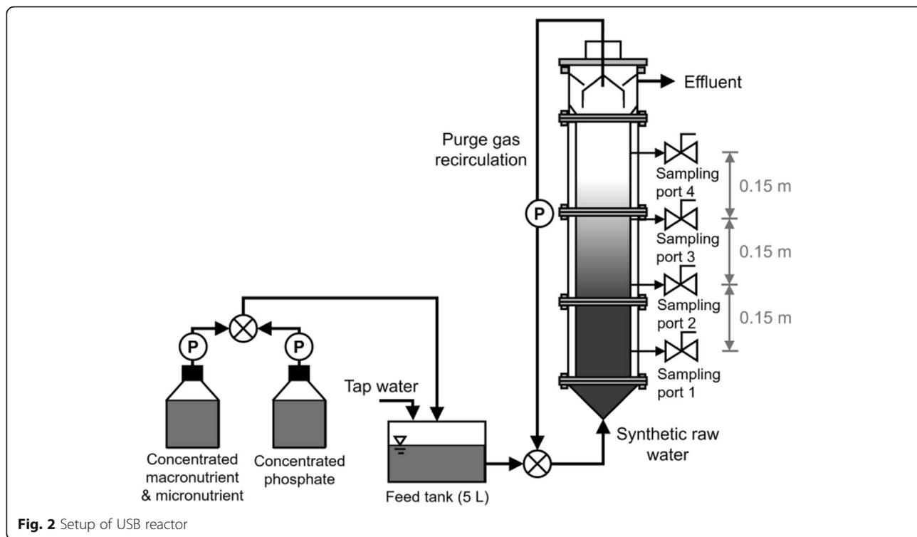
Fig. 2 Setup of USB reactor
