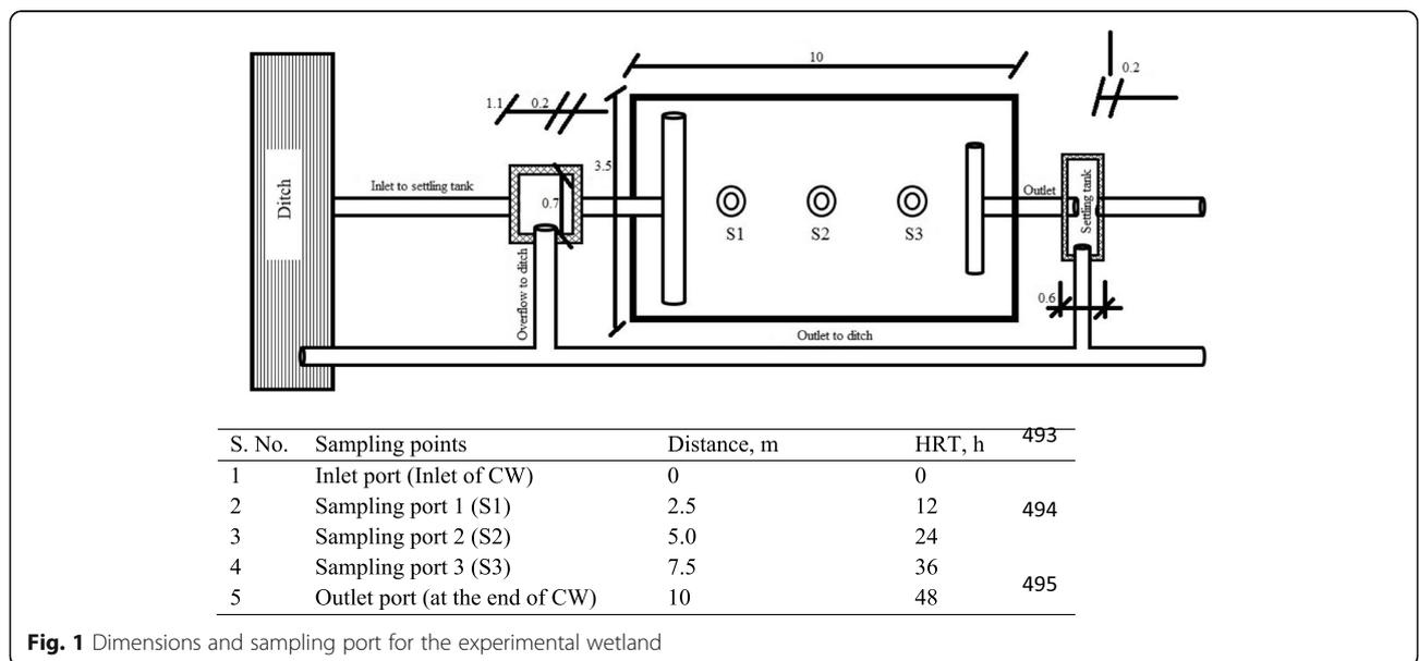
**Fig. 1** Dimensions and sampling port for the experimental wetland
