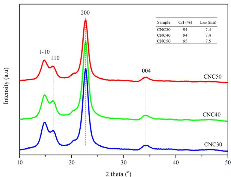
**Fig. 5** XRD patterns, crystallinity index and crystallite size of CNC30, CNC40, and CNC50
