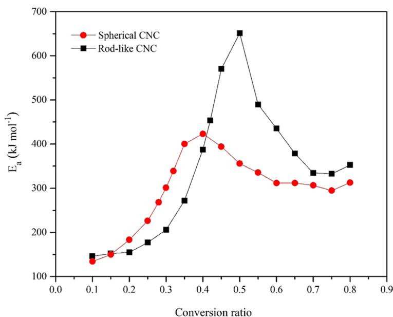
**Fig. 8** Activation energy versus conversion ratio for spherical CNC and rod-like CNC (CNC30)
