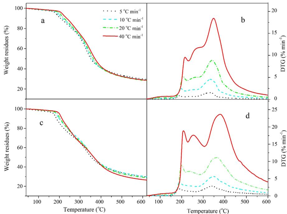
**Fig. 6** TG and DTG curves of spherical CNC (a, b) and rod-like CNC (CNC30) (c, d)
