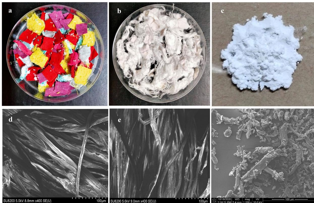
**Fig. 1** Photographs of CCW (a); TCC (b); MCC (c) and SEM images of CCW (400X) (d); TCC (400X) (e); MCC (1000X) (f)
