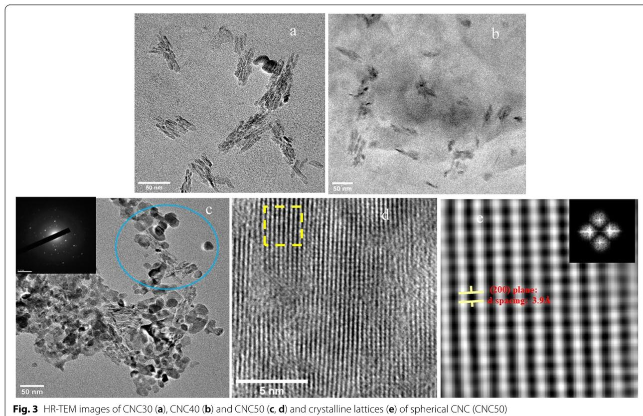
**Fig. 3** HR-TEM images of CNC30 (a), CNC40 (b) and CNC50 (c, d) and crystalline lattices (e) of spherical CNC (CNC50)
