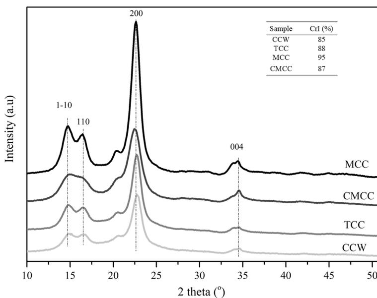
**Fig. 2** X-ray diffraction patterns and crystallinity index of MCC, TCC, CCW and CMCC
