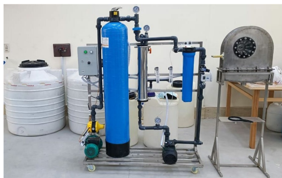
Fig. 1 Photograph of the investigated RO unit with ERS of Pelton Wheel
