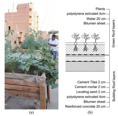
Fig. 7 a Soil-based green roof system [28], b Illustrative cross section for SD (authors)
