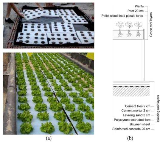
Fig. 9 a The DWC green roof system [29], b Illustrative cross section for DWC (authors)
