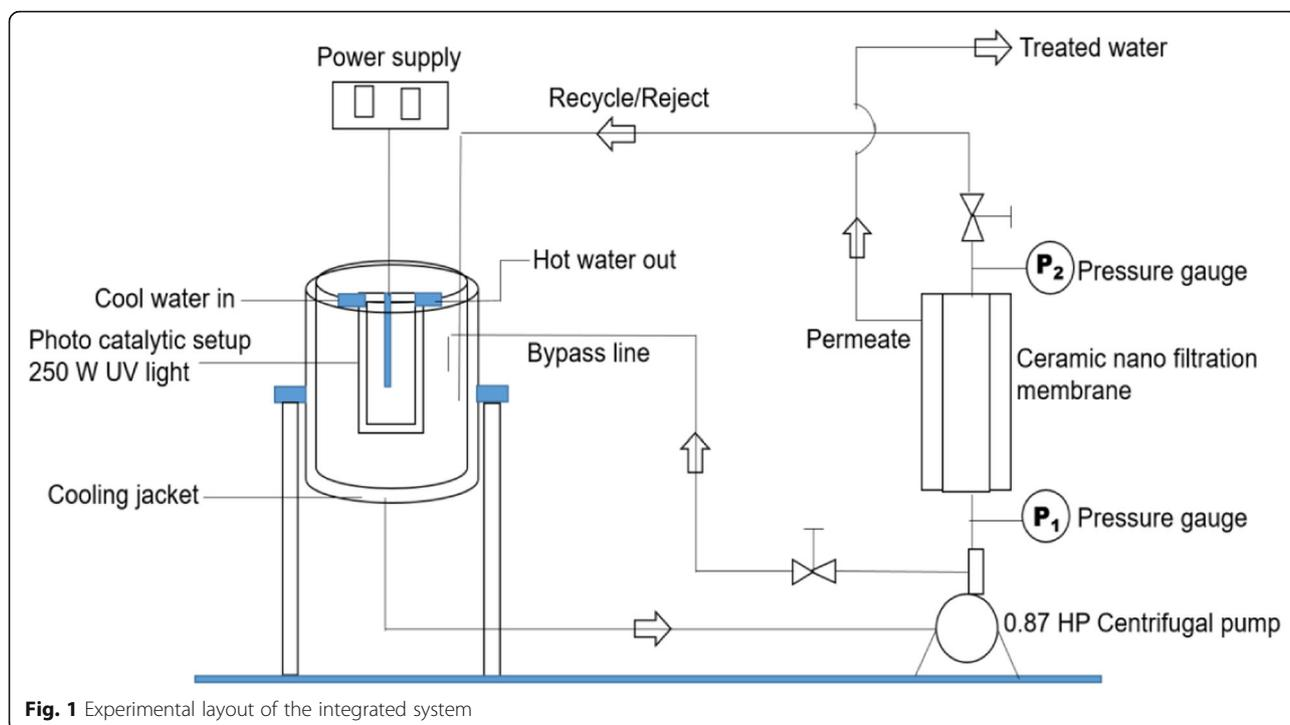
at the centre from the top side of the feed tank. Stainless steel (SS-316) was used in making the Photocatalytic reactor. Similar to the UV lamp, the feed tank also has a double jacket for the continuous supply of water to uphold the reactor temperature. The feed was pumped into the filtration membrane using 0.63 kW centrifugal pump.
