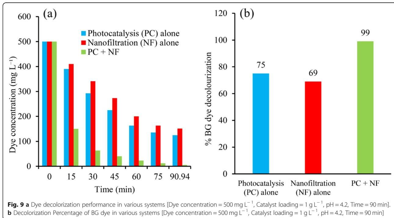
Fig. 9 a Dye decolorization performance in various systems [Dye concentration = 500 mg L<sup>-1</sup>, Catalyst loading = 1 g L<sup>-1</sup>, pH = 4.2, Time = 90 min]. b Decolorization Percentage of BG dye in various systems [Dye concentration = 500 mg L<sup>-1</sup>, Catalyst loading = 1 g L<sup>-1</sup>, pH = 4.2, Time = 90 min]
