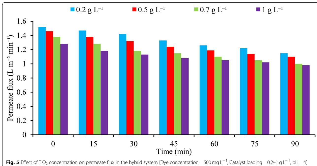
**Fig. 5** Effect of TiO<sub>2</sub> concentration on permeate flux in the hybrid system [Dye concentration = 500 mg L<sup>-1</sup>, Catalyst loading = 0.2–1 g L<sup>-1</sup>, pH = 4]
