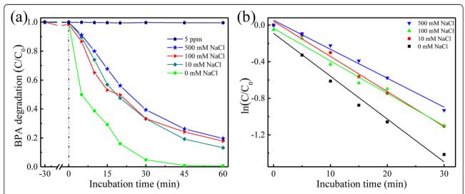
Fig. 4 (a) Effect of the NaCl concentration on the photocatalytic degradation of BPA with ZnO NPs under 365 nm UV light, (b) the plot of ln (C/Co) vs irradiation time for the photocatalytic degradation of BPA with ZnO NPs under different NaCl concentrations
