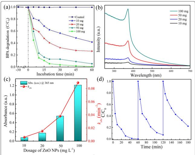
**Fig. 2** (a) Effect of the initial ZnO NPs catalyst loading (10–100 mg L<sup>-1</sup>) on the photocatalytic degradation of BPA (5 ppm) under 365 nm UV light (4×8-W tube light), pH 7 at room temperature, (b) full scan UV-visible spectra after different ZnO NPs loading, (c) linear relationship between ZnO concentration catalyst dose and UV absorption, and (d) reusability and stability test
