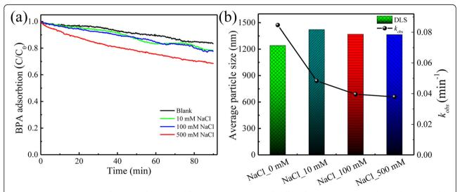
Fig. 5 (a) Sedimentation curve of ZnO NPs after loading different NaCl concentration, (b) effect of NaCl on average particle size distribution of ZnO NPs and the photocatalytic degradation rate constants
