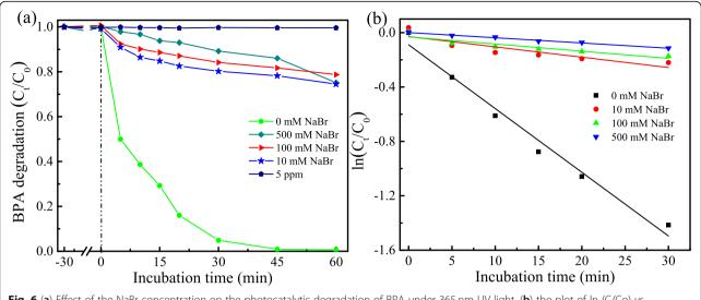
Fig. 6 (a) Effect of the NaBr concentration on the photocatalytic degradation of BPA under 365 nm UV light, (b) the plot of ln (C/Co) vs irradiation time for the photocatalytic degradation of BPA with ZnO NPs under different NaBr concentrations
