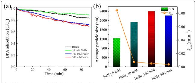
Fig. 7 (a) Sedimentation curve of ZnO NPs after loading different NaBr concentration, (b) effect of NaBr loading on average particle size distribution of ZnO NPs and the photocatalytic degradation rate constants
